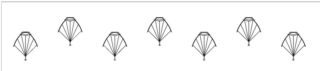
Such a farm will have a length toward the wave front of 3.9 km and will occupy 3.2 km<sup>2</sup>. The rated power relative to the use of sea will thus be 15.3 MW/km<sup>2</sup>.
