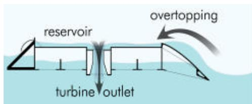
It is very simple: The Wave Dragon™ overtopping device elevates ocean waves, and the water overtopping Wave Dragon™ is stored temporarily in a large reservoir creating a head, i.e. the difference between the "normal" level of the water surface and the water surface in the reservoir. This water is let out of the Wave Dragon™ reservoir through several turbines, thus generating electricity like in hydro power plants.
